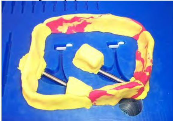
Figure 9. Sacrificial material (yellow), support material (blue) and embedded components [10].
