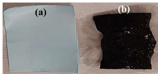
Figure 2. Digital images of PVA-Co nanofiber, (a) after spinning, dry form, (b) reduced with \text{NaBH}_4 , wet form.
