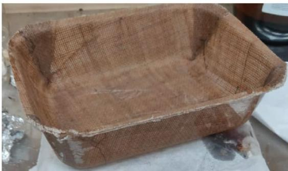
Figure 3. natural fibre reinforced polymer composite tray from vacuum bagging
