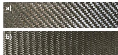
Figure 2. The composite samples a) 0/90, b) -45/+45 fiber orientation.
