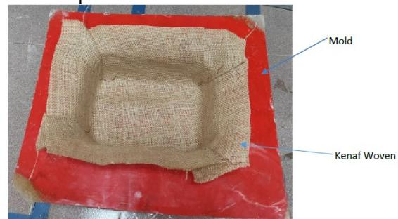
Figure 2. kenaf woven fibre with mold
