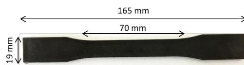
Figure 1. Dog bone tensile test sample.
