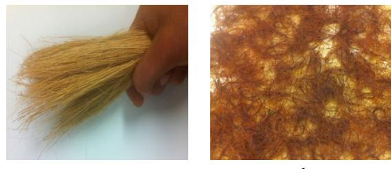
Figure 1. Date palm fibers preparation, a. PDPFiber after extraction, b. PDPFiber after treatment
