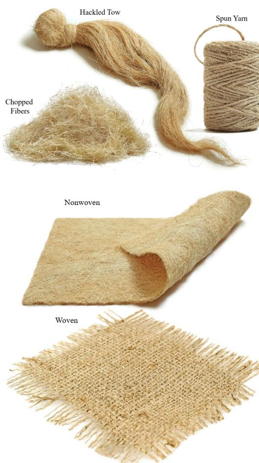
Figure 2. Different textile forms of PalmFil fibers <sup>4</sup>
