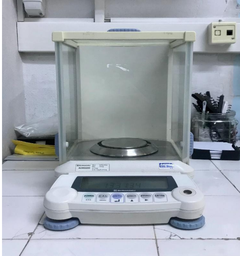
Hassas Terazı (Shimadzu, AUV220D)
