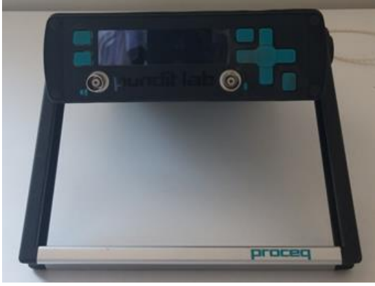
UPV Cihazı TS EN 12504-4; ASTM C 597-02; BS 1881 Part 203; ISO1920-7:2004; IS13311; CECS21
