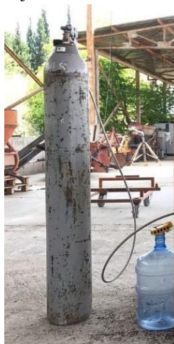
Figure 2. NH 3 , regulator and pipe.
