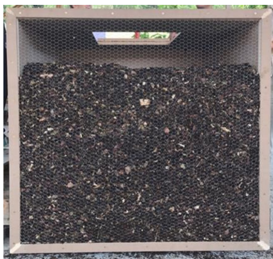
Figure 7. Biofilter with biofilter material.
