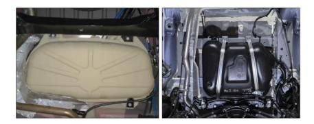
Figure 17. Assembling methods of fuel tanks to the underbody
