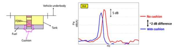
Figure 11. Effect of cushion addition between FDM & tank bottom
