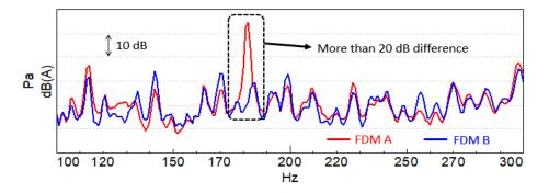
Figure 7. Frequency spectra for the noisy and the silent FDMs
