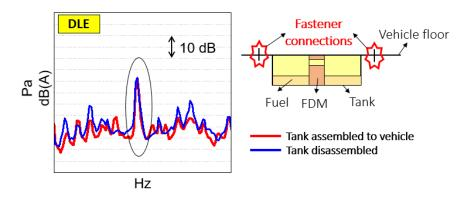
Figure 18. The effect of disassembling the fuel tank from the vehicle body
