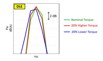
Figure 12. Effect of Flange Fastening Torque Value
