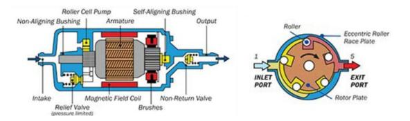
Figure 4. Internal structure and operation principle of a roller-cell type of fuel pump
