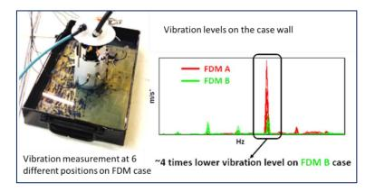
Figure 8. Vibration levels on the cases of the two FDMs on bench
