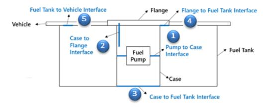
Figure 5. Schematic of the FDM-Fuel Tank-Vehicle Group
