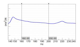
Figure 13. FRF Measurement result on the case wall of FDM A
