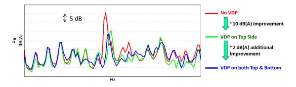
**Figure 15.** Improving effect of the VDP applications on the noise level (measured at DLE on the vehicle).
