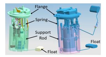
Figure 9. Structure of the two FDM units
