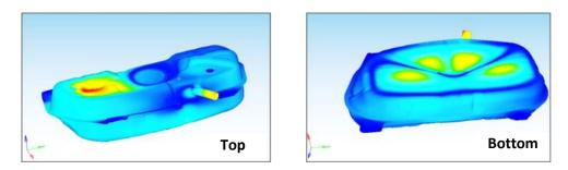
Figure 14. Two structural modes of the fuel tank (top and bottom) close to the rotational frequency of the FDM pump.
