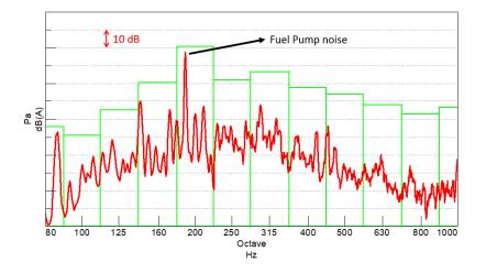
Figure 3. The frequency spectrum of noise measured by the microphone at the DLE.
