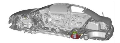
Figure 16. Location of a fuel tank on a passenger car
