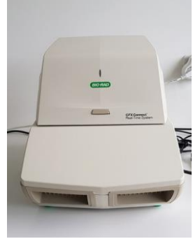
QPCR (Bio-Rad CFX Connect)
