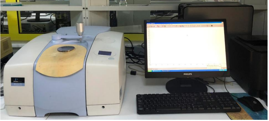
Infrared Spektrofotometresi (IR) (Pekin Elmer, Spectrum 100)
