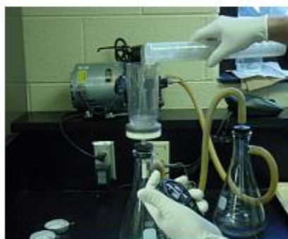
Membrane filter apparatus
