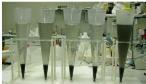
Figure 4. Procedure chart for settleable solids determination
