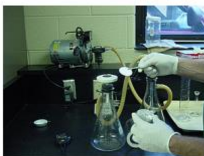
Place filter on the membrane filter apparatus
