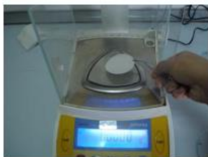
Weigh 0,45 \mu\text{m} membran filter
